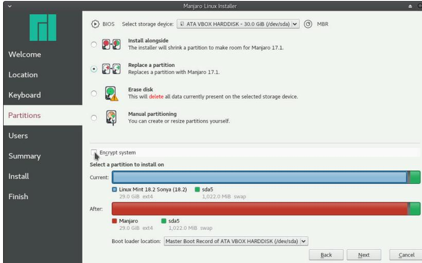
9: In all assisted installation options (*Install alongside, Replace a partition* and *Erase disk*), a checkbox above the two status bars enables you to automatically encrypt your system during the installation. Tick it to enable encryption.
